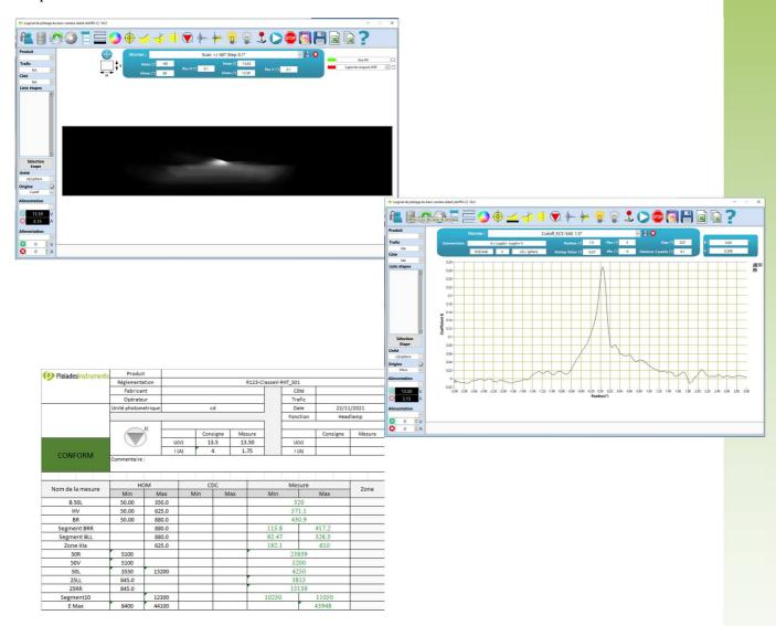
This software allows a large type of measurements for complex analysis, production... A database of standards that can be tested is provided with the system. ALPES-C provides a report indicating if a measurement is conform to the standards. Moreover, lots of measurement types are available: point, scan, cut, succession of measurements on the same products and cutoff stability.
